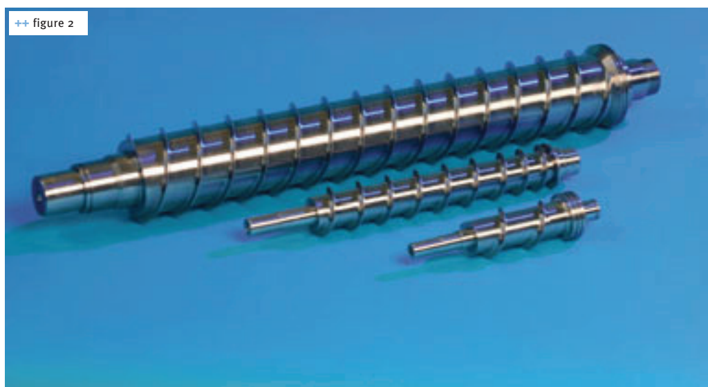
++ figure 3 Shaved ice and StreamIce are made by a conveying screw that scrapes frozen water from the walls of a freezing cylinder. The ice is then compacted and transported to the discharge. The size of the discharge opening defines the particle size of the ice
